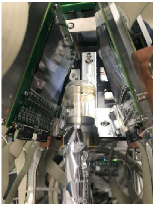
Cocotier LH2 target with FOOT Si-trackers as subsystem of the CALIFA calorimeter
