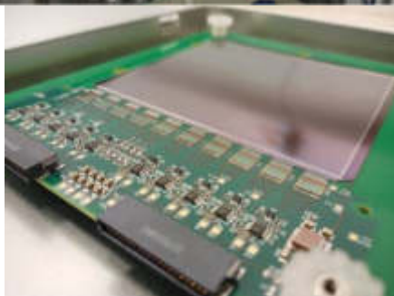
Si microstrip vertex tracker assembled for 2022 FAIR Phase-0 beam time
