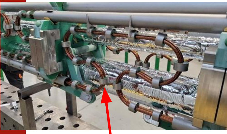
Bus Bars thermal compensation loop
