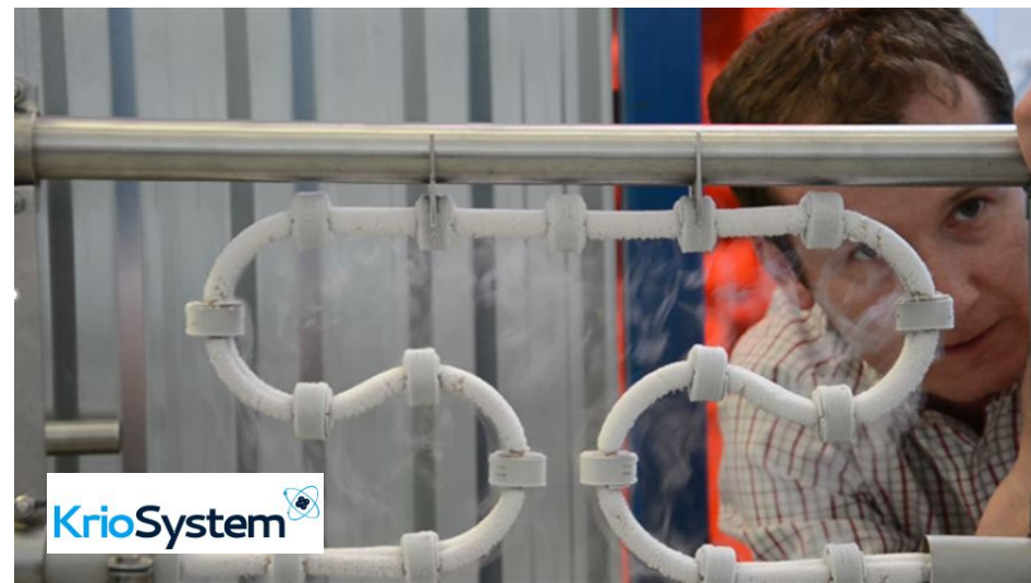
Bus Bar compensation loop tests at liquid nitrogen
