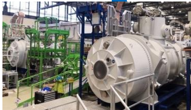
SFRS: Multipllett-Magnet in teststand@CERN
