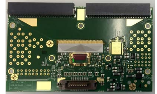
Radiation test of FEB-C and test of conductive glue
