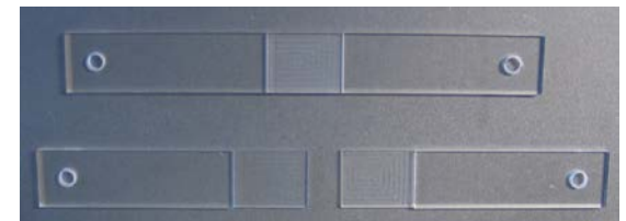
Pulltest samples (behaviour of silver conductive glue)
