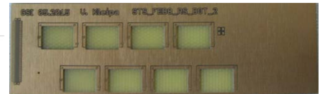
Pulltest samples (behaviour of silver conductive glue)
