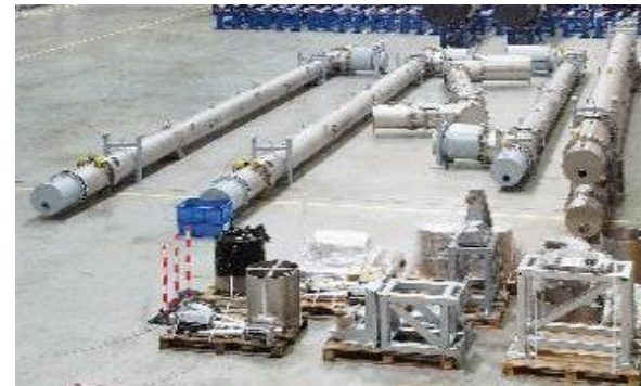
SIS100: Cryo Bypass Lines by company Kriosystem
