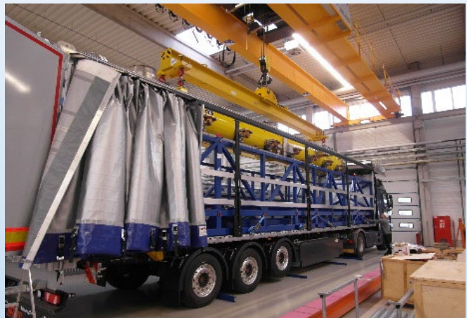
Unloading of the cryomodule after transport
